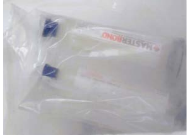
Master Bond fluids were shipped frozen and after thawing offered 6-8 hours of working life.
