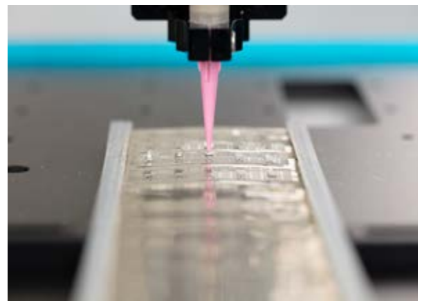
The combination of Master Bond's EP3HTSDA-2Med epoxy and Nordson EFD's precision dispensing system delivered a robust, repeatable process for manufacturing this critical surgical LED die attach component.
