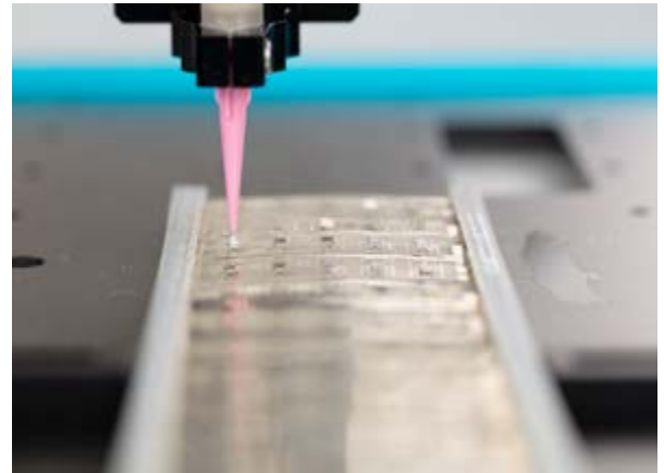
The 20-gauge rigid tapered tip was selected to manage backpressure issues, and reduce flow restriction during dispensing.
