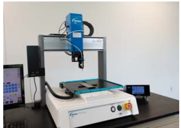
The engineering team selected the 3-axis PRO4 automation system and UltimusPlus I dispenser because it delivered the consistent, precise process control necessary for the application.
