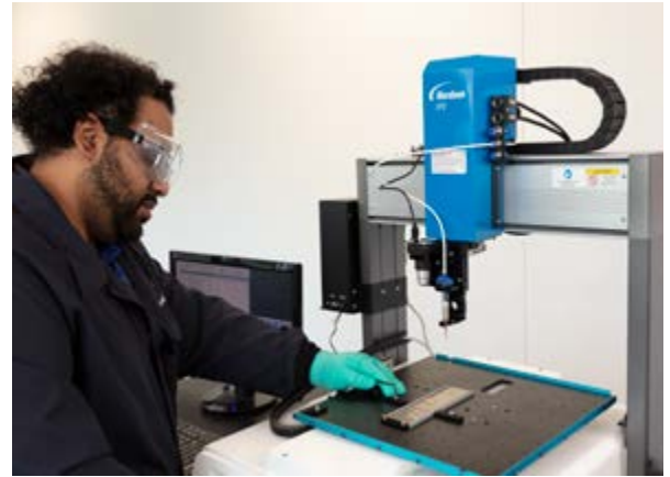
The Nordson EFD fluid dispense solution for the application included a 3-axis PRO4 tabletop robot, an UltimusPlus I dispenser, a 3cc syringe barrel, and a 20-gauge rigid tapered tip.
